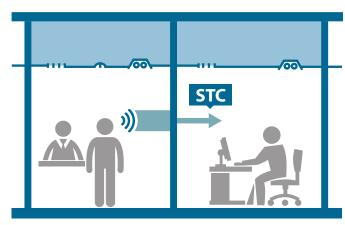
Meet sound blocking requirements between rooms by using full-height walls or lightweight plenum barriers.
