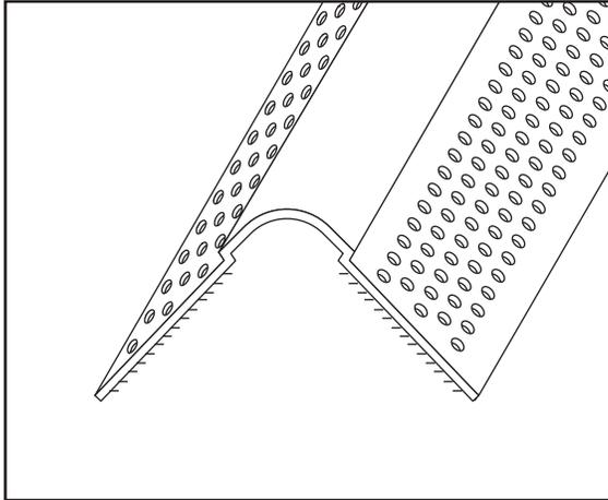
**Description:** Trim-Tex Mud Set 350 Bull Corner Bead is designed to finish outside 90° drywall corners and provide a soft, rounded look. It is installed and bonded to the drywall with drywall compound.
