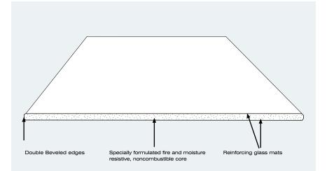
GlasRoc\* Shaftliner is a 1" (25.4 mm) thick gypsum board with a specially formulated, fire resistive, non combustible core combined with reinforcing glass mats and double beveled edges for ease of installation.
