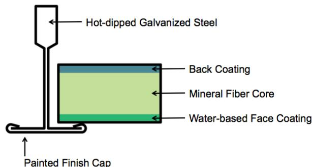
USG Ceilings™ Brand: Eclipse™ ClimaPlus™, Eclipse™ ClimaPlus™ HRC, Eclipse™ ClimaPlus™ Firecode®, Astro® ClimaPlus™ X-Technology Wet Felted Mineral Fiber Ceiling Panels
