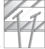
joists that are 16" (406 mm) o.c.,  $\frac{1}{2}$ " (12.7 mm) or  $\frac{5}{8}$ " (15.9 mm) DensArmor Plus panels may be applied.
