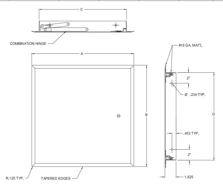
STANDARD FEATURES: SLOTTED SCREW CAM LATCH, CARBON STEEL, PRIME COAT BAKED ENAMEL FINISH OPTIONS:
