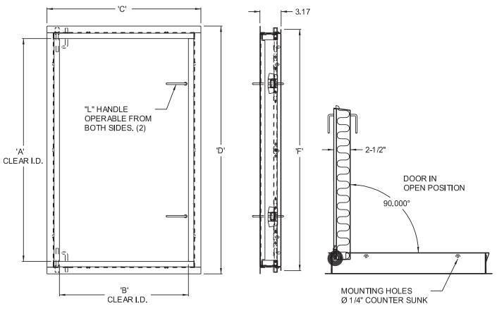
STANDARD FEATURES: UNIVERSAL SELF LATCHING BOLT- OPERATED BY "L" HANDLE ON BOTH SIDES. COIL SPRINGS TO CONTROL OPENING AND CLOSING
