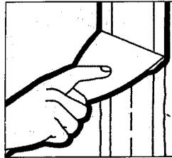
firmly along joint to tightly embed tape. Do this in both directions, removing excess compound by holding the knife at a 45° angle to the panel
