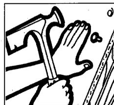
by the last blow of the drywall hammer. Drive nails in straight, do not over drive or countersink nails. This results in breaking the face paper or fracturing the gypsum core. Double-nailing reduces the likelihood of nail pops. (It is highly recommended for ceilings.) Drive the first nails 300 mm (12") on centre along framing and the centre or field of board and second nails about 50 mm (2") from the first. Fasten the perimeter 180 mm (7") o.c. for ceilings and 200 mm (8") o.c. for walls.
